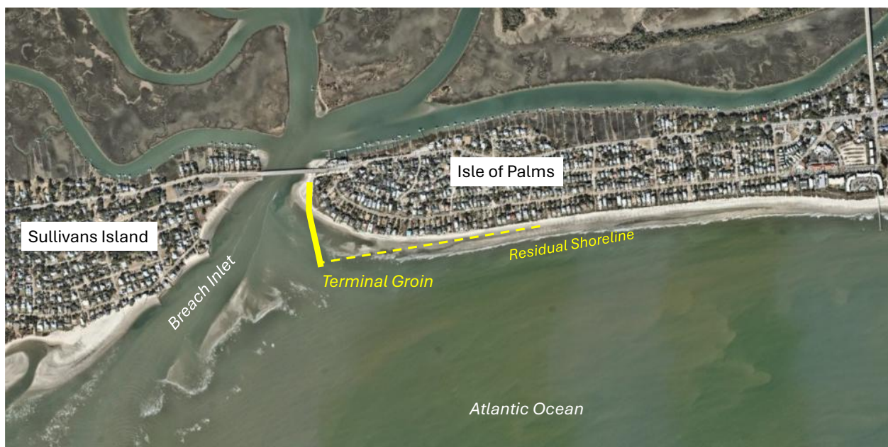
Figure 13: CONCEPT of a long terminal groin and the intended residual beach position response at the southern end of IOP adjacent to Breach Inlet.
