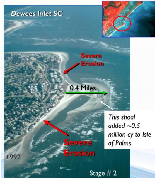
Figure 5: Example of shoal attachment event along northern end of Isle of Palms and the associated severe erosion along the shoreline leeward of the shoal edges (CSE, 2024b).
