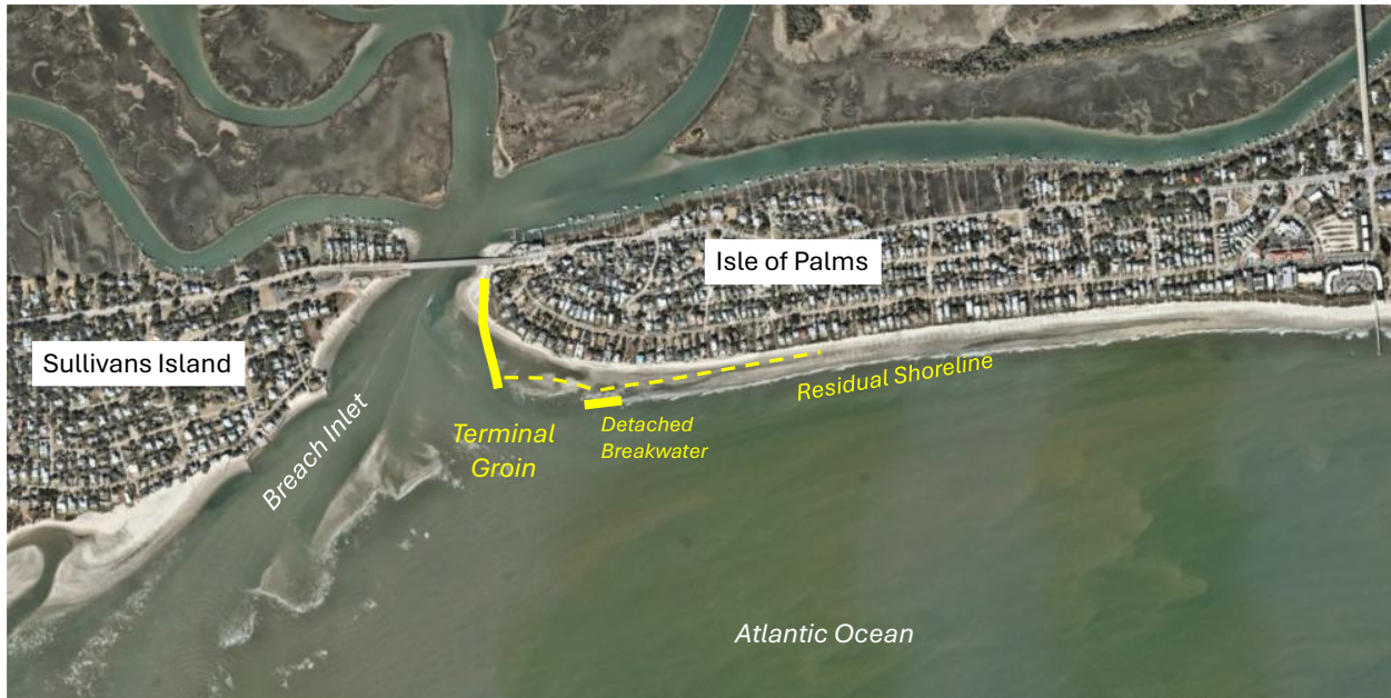
Figure 14: CONCEPT of a short terminal groin and updrift detached breakwater to address the natural curvature of the island’s southern shoreline. The CONCEPT of residual beach position response to both the short terminal groin and updrift breakwater at the southern end of IOP adjacent to Breach Inlet is also depicted in the figure.
