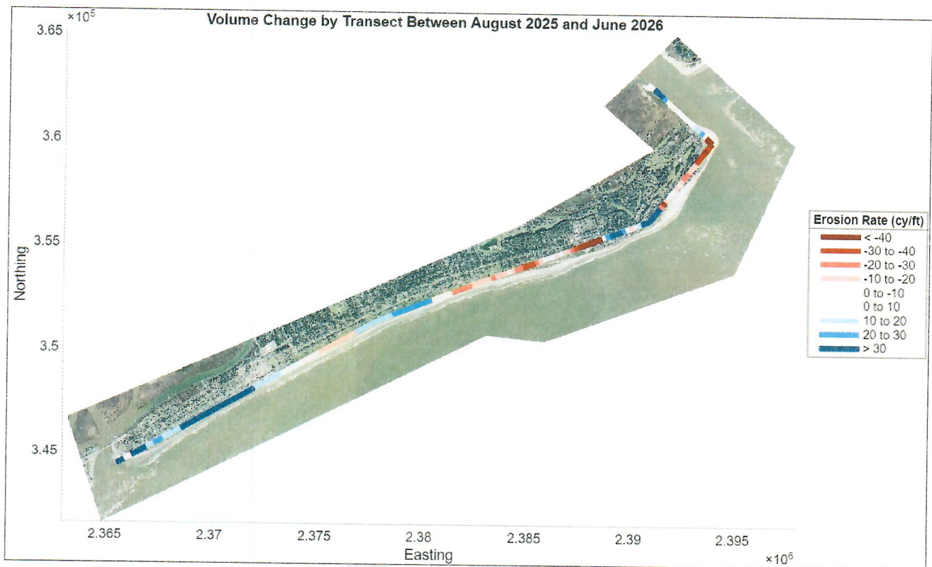
FIGURE B. Image showing the volume change by station for the year. Accretion (blue) is mostly seen in the south end of the island, where the USACE project and downdrift movement of sand have built up the beach. There are also pockets near the shoal attachment areas. There is erosion (Red) shown in some of the erosion hotspots in reaches 5 and 6.
