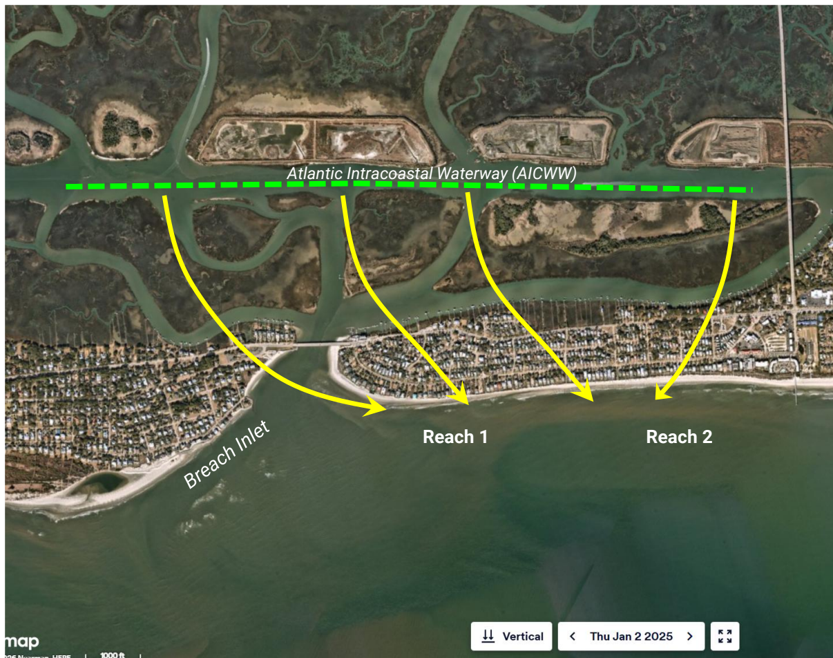
Figure 5-7: Breach Inlet AICWW Maintenance Dredging Sand Alternative showing the assumed maintenance dredging sand source within Breach Inlet and conceptual placement along Reaches 1 and 2.
