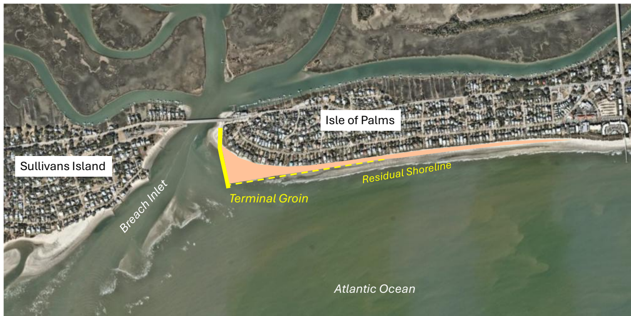
Figure 5-8: Conceptual terminal groin alternative at the southern end of Reach 1 adjacent to Breach Inlet.
