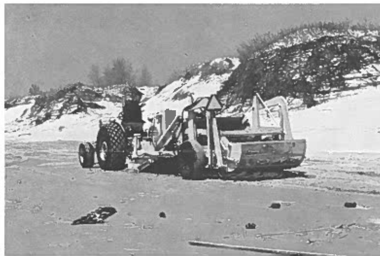
BeachLeach is tractor-towed by unit with high flotation tires, and is designed to process very wet sand.
